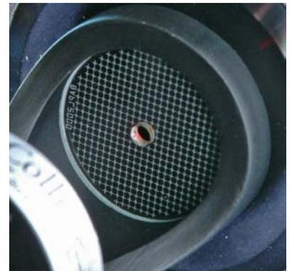
Tilt the main mirror with the help of the adjustment screws until the laser beam passes through the hole (and is reflected into itself).
