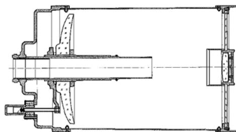
Simplified sketch of the SC-secondary mirror tilting mechanism. Three screws are arranged 120° apart, around a center pin on which the secondary mirror pivots. Loosening one screw and tightening another will tilt the mirror into the designed position.
