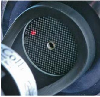
If you see this on your reference plane, adjust (tilt) your main mirror in a way that the laser point passes exactly through the center hole thus being reflected into itself.
