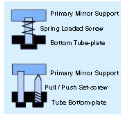
On most larger Newtonians, 3 pairs of push/pull screws are used (lower sketch). In the lower sketch the left side screw is threaded into the mirror support plate and will pull that side down, the right hand screw has it's thread cut into the bottom plate and would lift the mirror up.
