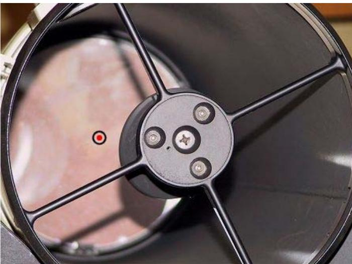
Most telescope constructions adjust the secondary mirror by three loaded screws like those (allen head screws) shown here in the picture. In other words: Turn one screw slowly clockwise and the secondary mirror is tilted in the direction towards this screw. When the laser's light point is centered correctly in the marker circle, successful adjustment of the secondary is achieved.
