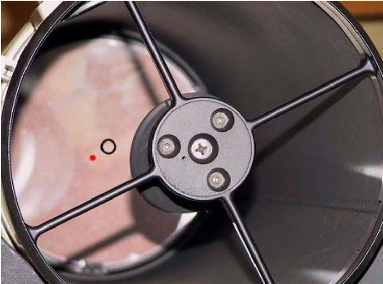
**Picture 1 left** shows the laser beam (red dot) obviously missing the marker circle in the center of the main mirror. Note the three adjustment Hex head screws of the secondary mirror spread 120° apart. Very cautiously and only in small steps re-tilt the secondary mirror by very slowly tightening and releasing these adjustment screws. While you look directly onto the main mirror watch the laser's light dot moving into the center marker circle while you are adjusting the secondary.
