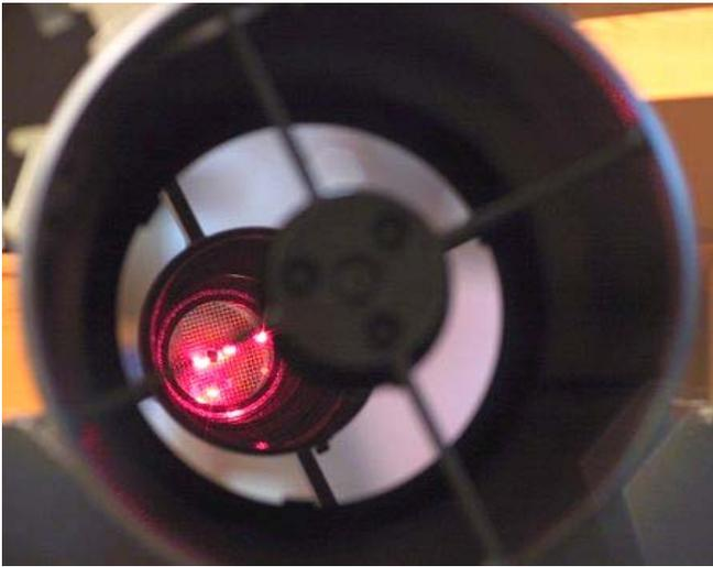
**Picture above** again shows the view from the tube's front to the reflected images of the secondary mirror and the grid plane.
