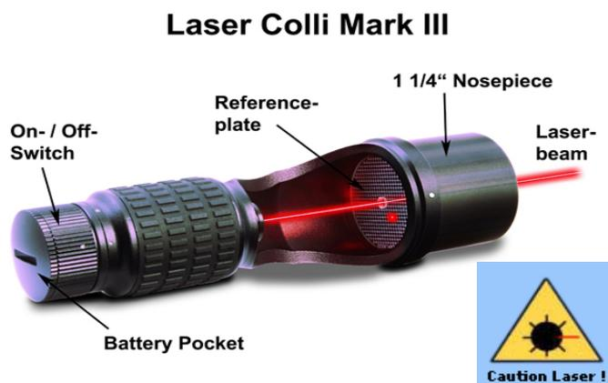
Of course, the **Laser-Colli™ Mark III** functions reliably only if the laser beam itself leaves its own housing in an absolutely centered position.
