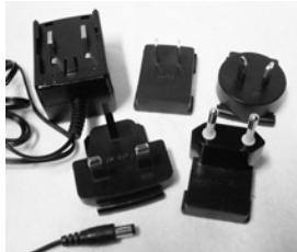
Plug the socket of the AC Adapter into the back of the Receiver unit (shown in bottom right image below). Then install the plug required for your location (four plugs are supplied-USA/Europe/UK/Australia).
