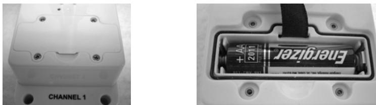
Remove the four small screws (shown in above image) from the door of the Anemometer with a small screwdriver. Insert two AA batteries (user supplied) as indicated in the sensor (see right image above). Replace the door of the Anemometer by installing the four small screws to hold it in place.
